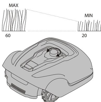
For the first few weeks of mowing, set the cutting height to 60 mm to avoid cutting the boundary wire and guide wire. Lower the setting one step each week thereafter until the desired cutting height is reached.
