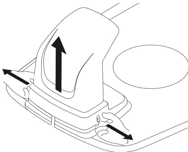
Remove the protective cover on the charging station by pressing in the tabs on each side of the base and lifting away the cover.
