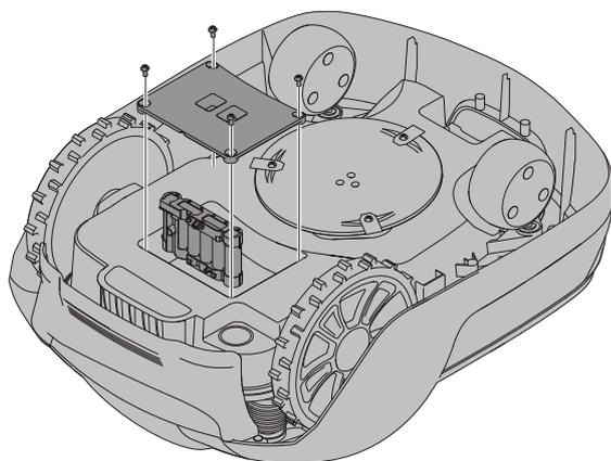
**WARNING!** Press the **STOP** button and remove the safety key before replacing batteries and wear protective gloves.
